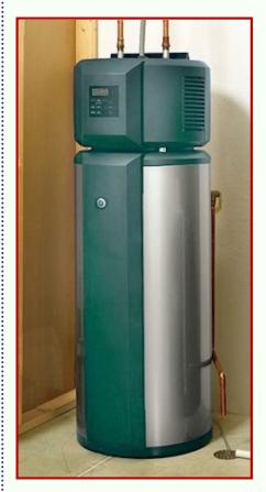
Stand-alone heat pump water heaters require installation in locations that remain between 40 to 90 degrees Fahrenheit and provide at least 1,000 cubic feet of air space around the unit. Cool exhaust air can be exhausted to the room or outdoors. Installation in spaces with excess heat, such as furnace rooms, works best. Heat pump water heaters will not operate efficiently in a cold space,
