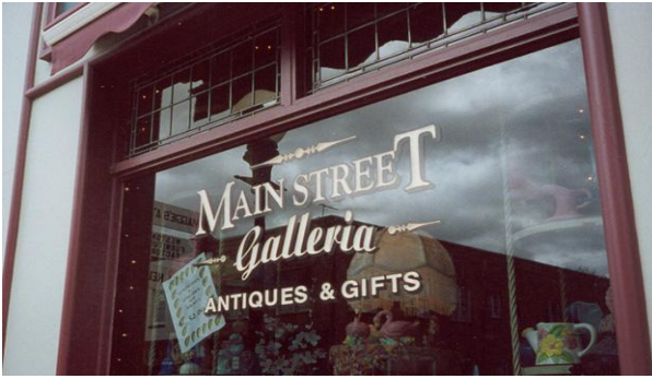
Example of a storefront display window sign. This sign is a laser cut vinyl decal that is adhered to the window.
