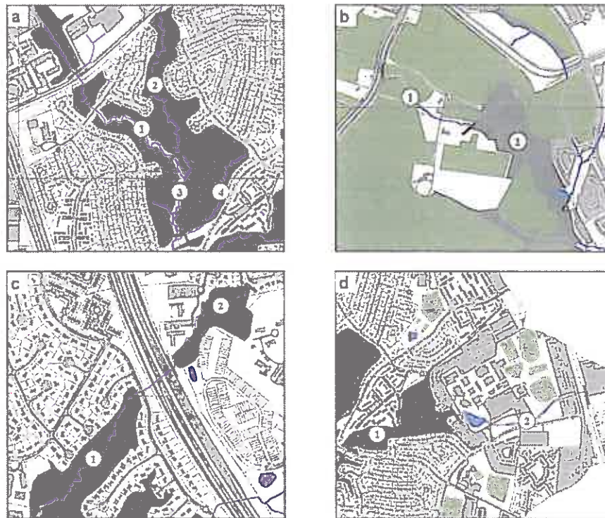
Figure 21: Various physical factors control how survey reaches are delineated. (a) Survey reaches based on the confluence of stream tributaries. (b) A long tributary split into ¼ mile survey reaches.
