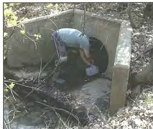
Figure 30: Measuring flow (as volume per time)
