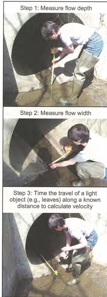
Figure 31: Measuring flow (as velocity times cross-sectional area)
