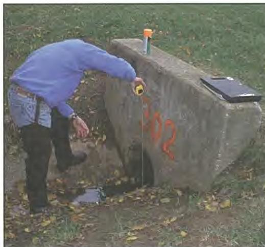
**Figure 27: Measuring Outfall Diameter**
