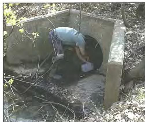
Figure 30: Measuring flow (as volume per time)
